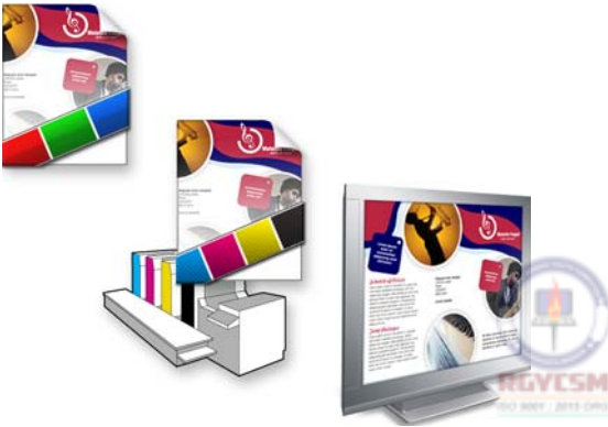
Top left: An RGB color profile is assigned to the document. Middle and right: Assigning a specific CMYK profile allows an on-screen simulation of the printed output.
